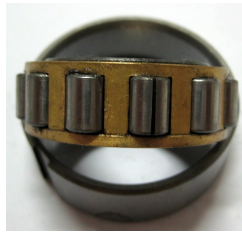
b) Rolling element fault
