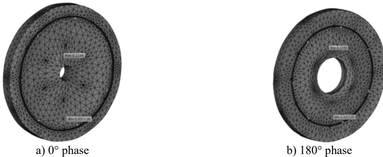
Fig. 3. Simulation of eigenfrequency of the circular waveguide
