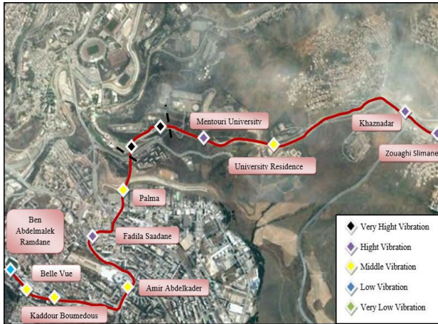
Fig. 6. The level of vibration inside the Constantine's tramway
