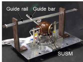
**Fig. 3.** Experimental apparatus of SUSM for space
