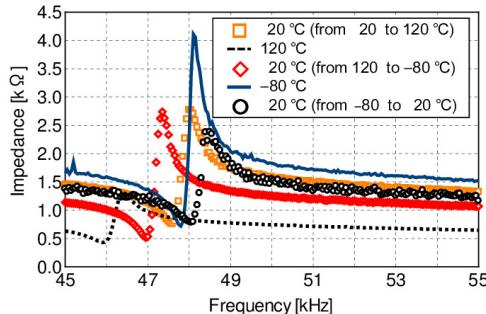
**Fig. 6.** Impedance characteristics in temperature cycle
