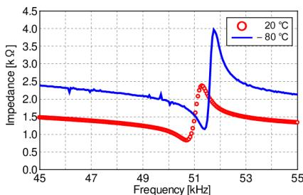
**Fig. 4.** Impedance characteristics at  $20^{\circ}\text{C}$  and  $-80^{\circ}\text{C}$
