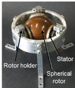
**Fig. 1.** Schematic of SUSM
