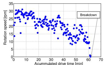
**Fig. 5.** Rotation speed of SUSM at  $-80^{\circ}\text{C}$
