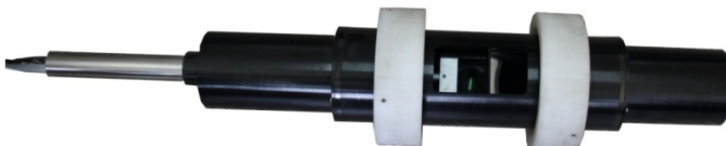
Fig. 1. Intelligent bore peek and measurement system based on machine vision technology for gun barrel
