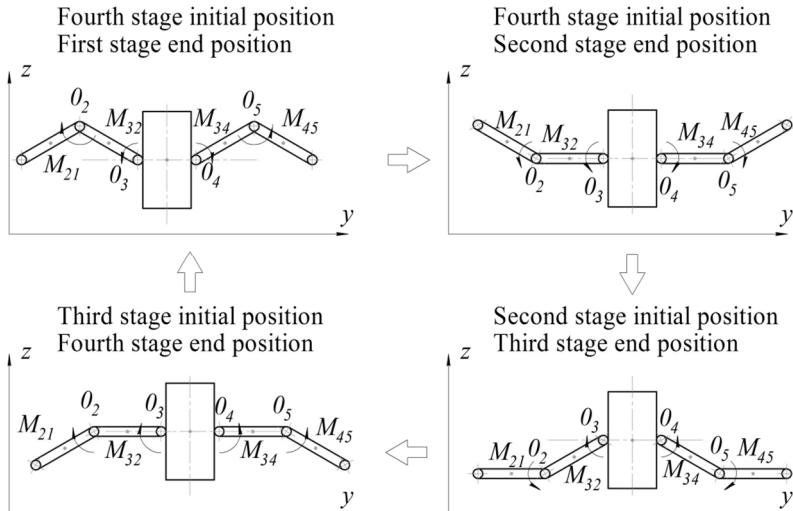
Fig. 4. Sequence of the stages of motion of the links of the mechanical system as an ornithopter
