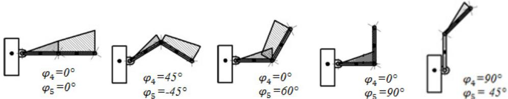
Fig. 2. Diagrams of distribution of forces of resistance along the lengths of the links 4 and 5
