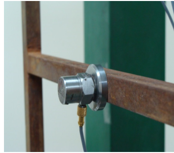
Fig. 4. The connection of the accelerometer to the structure
