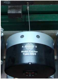
Fig. 3. The electrodynamic shaker and stinger
