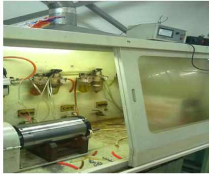
Fig. 4. Experiment table of rotor vibration
