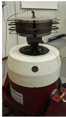
Fig. 4. Arrangement of technical experiment for a determination of the dynamic characteristic of rubber element
