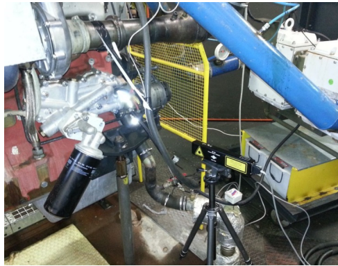
Fig. 6. Measurement of crankshaft pulley angular vibrations
