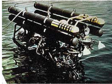
Fig. 5. Cable-controlled undersea recovery vehicle CURV
