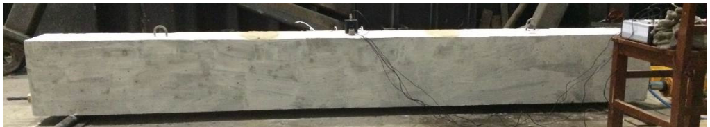
Fig. 3. The experimental process of the pre-stressed concrete beam
