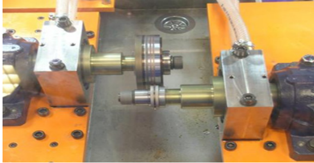
Fig. 1. RoR Tribometer and test configuration
