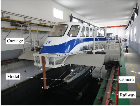
Fig. 3. Towing carriage facility
