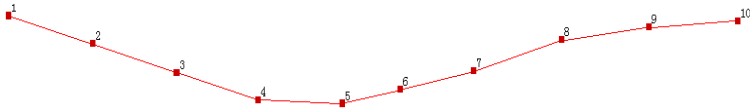
Fig. 14. The first order frequency and modal shape of experimental test (Mode 1: 36.4213 Hz, 0.11 % AMPS)
