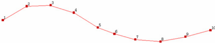
Fig. 12. The second order frequency and modal shape of experimental test (Mode 2: 130.5435 Hz, 5.87 % AMPS)
