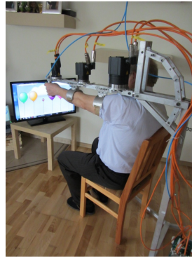
Fig. 2. Prototype of ELISE robot for spastic upper limb rehabilitation
