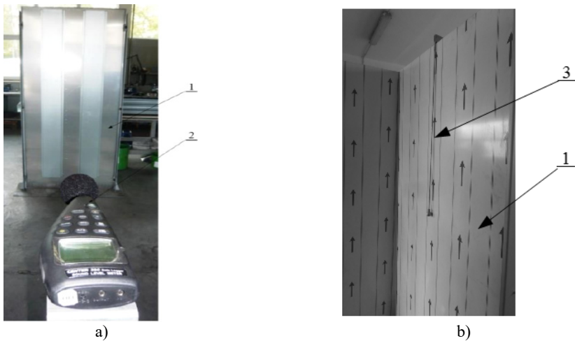
Fig. 3. Measurements test bench a) the back side of the wall b) the front side of the wall 1 – panel construction, 2 – sonometer, 3 – a metal impactor
