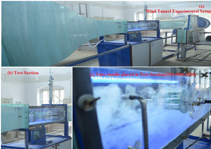
Fig. 1. Wind tunnel test experimental setup
