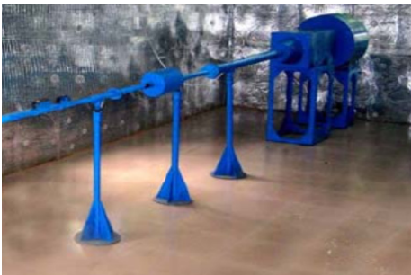
Fig. 10. Transmission loss experiment of the muffler
