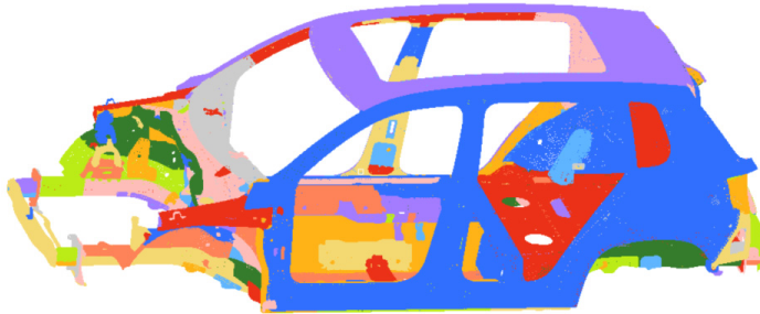
Fig. 1. The finite element model of body in white
