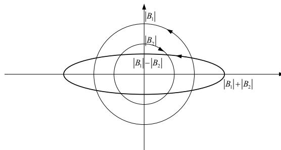
Fig. 3. Synthesizing diagram of shaft center orbit
