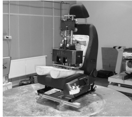
Fig. 5. Testing car seat with 2H dummy
