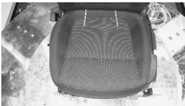
Fig. 7. Location acceleration sensors
