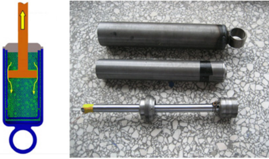
Fig. 2. MR damper schematic diagram and physical contrast diagram
