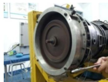
Fig. 2. Thick turbine casing single-point rubbing experiment
