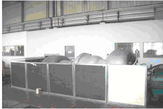
Fig. 2. The layout of the sound-absorbing panels surrounding the turbocharger
