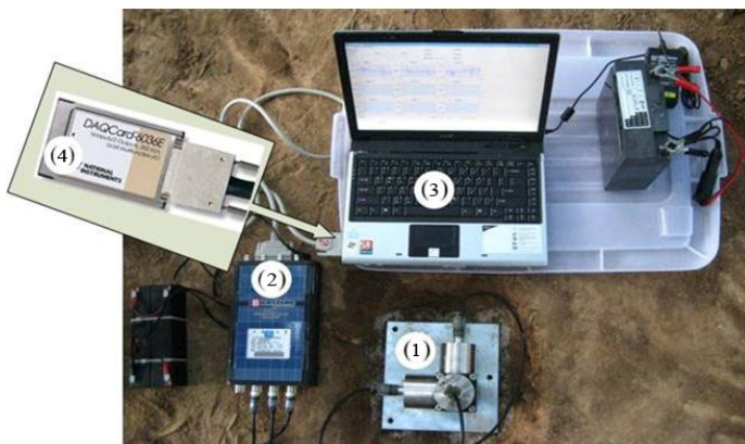
Fig. 2. Measuring equipment: (1) accelerometers, (2) integrator, (3) and (4) data acquisition system
