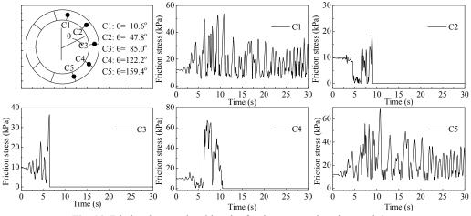
Fig. 14. Frictional stress-time histories for the concrete interfaces at joints
