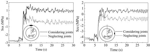
a) Horizontal stress in the section located at  $\theta = 0^{\circ}$  b) Vertical stress in the section located at  $\theta = 90^{\circ}$ Fig. 12. Stress in concrete time histories
