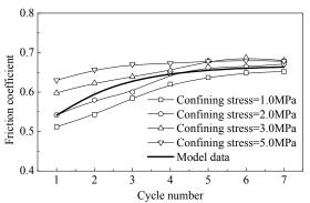
Fig. 5. Variation of average friction coefficient with cycle number
