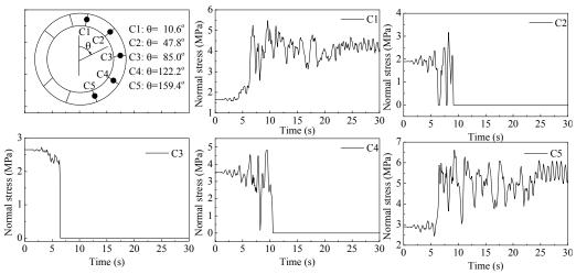
Fig. 13. Normal stress-time histories for the concrete interfaces at joints
