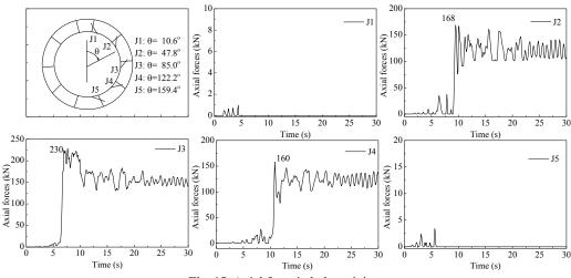
Fig. 15. Axial force in bolts at joints
