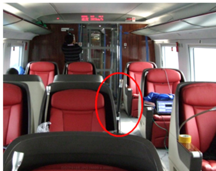
Fig. 17. Testing point of noise in the front part for the high-speed train
