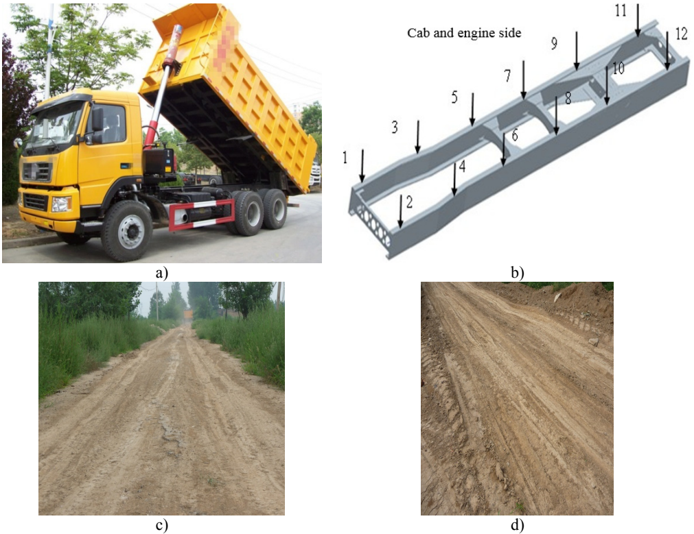
Fig. 5. The operation modal test of heavy duty truck and the surface of test road
