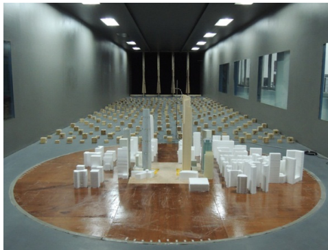
Fig. 10. GZET model in wind tunnel tests
