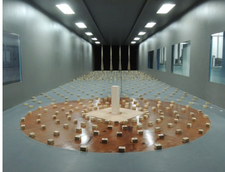
Fig. 1. The CAARC building model in wind tunnel tests
