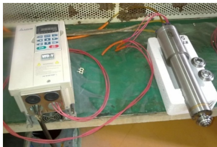
b) Motorized spindle was driven by inverter
