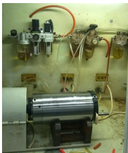
a) The motorized spindle used oil and gas lubricating system during operation
