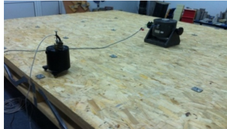
Fig. 6. Experimental test in the second methodology (forced vibrations)
