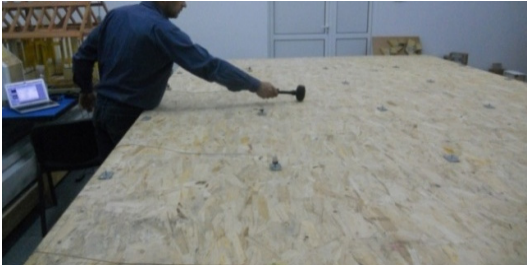
Fig. 5. Experimental test in the first methodology (free vibrations)
