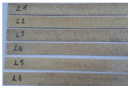
Fig. 3. Produced bio-composite beams
