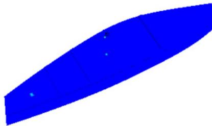
**Fig. 7.** Dynamic stress distribution of lateral plates after optimization
