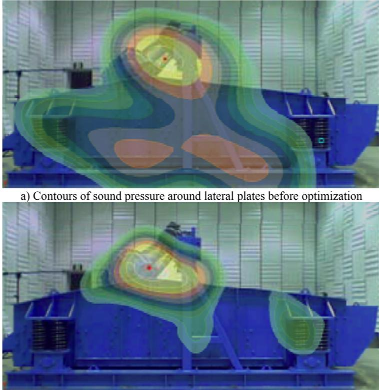
**Fig. 11.** Contours of sound pressure around lateral plates before and after optimization
