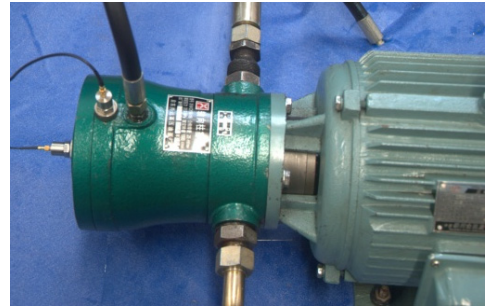
Fig. 7. The hydraulic piston pump experiment system
