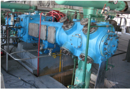
a) The tested reciprocating compressor
