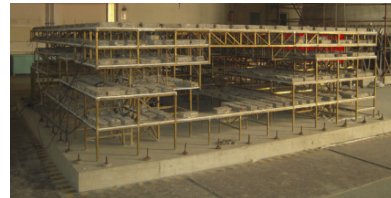
Fig. 2. The schematic photo of the structure shaking table model
