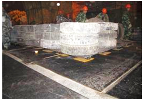
d) Composite protective structures of steel-rubber tires
