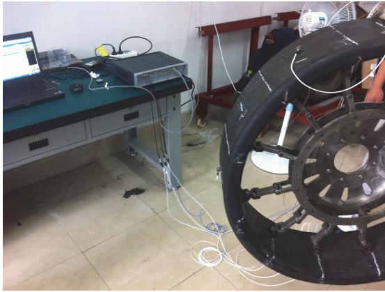
Fig. 7. Vibration modal test
