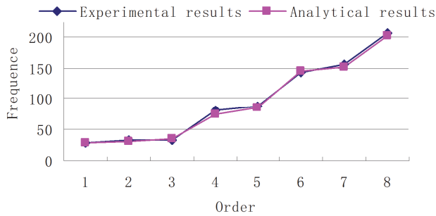
Fig. 9. Vibration frequency comparison of the experiment and theory
