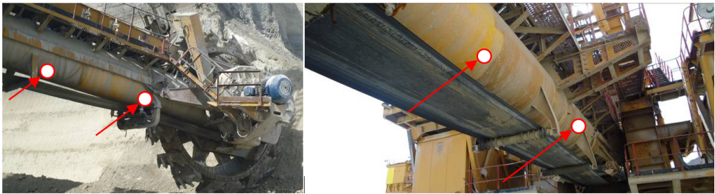
Fig. 5. Location of the acceleration measurement points on the boom
