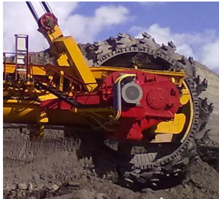
Fig. 7. New drive of the bucket wheel excavator ER1250 operating body
