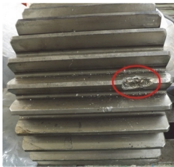
Fig. 19. The damaged planetary gear of the wind turbine gearbox
