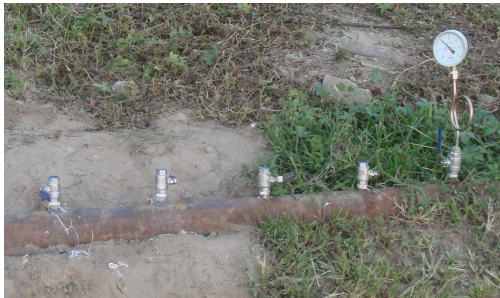
Fig. 8. Experiment schematic of simulated leaks with different apertures
