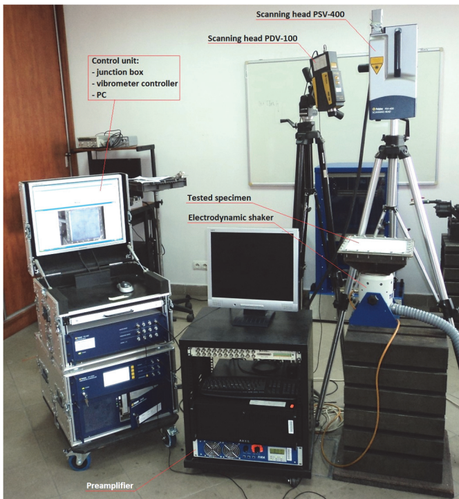
Fig. 1. Experimental setup during the modal analysis
