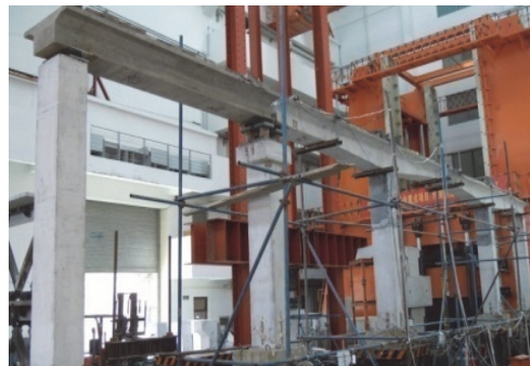
Fig. 2. The 1/10 scaled bridge model
