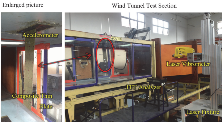
Fig. 6. Wind tunnel test setup
