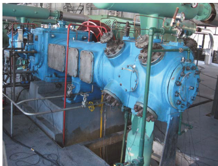
Fig. 6. Experimental equipment of reciprocating compressor
