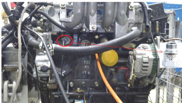
Fig. 3. IC engine with location of mounted sensor
