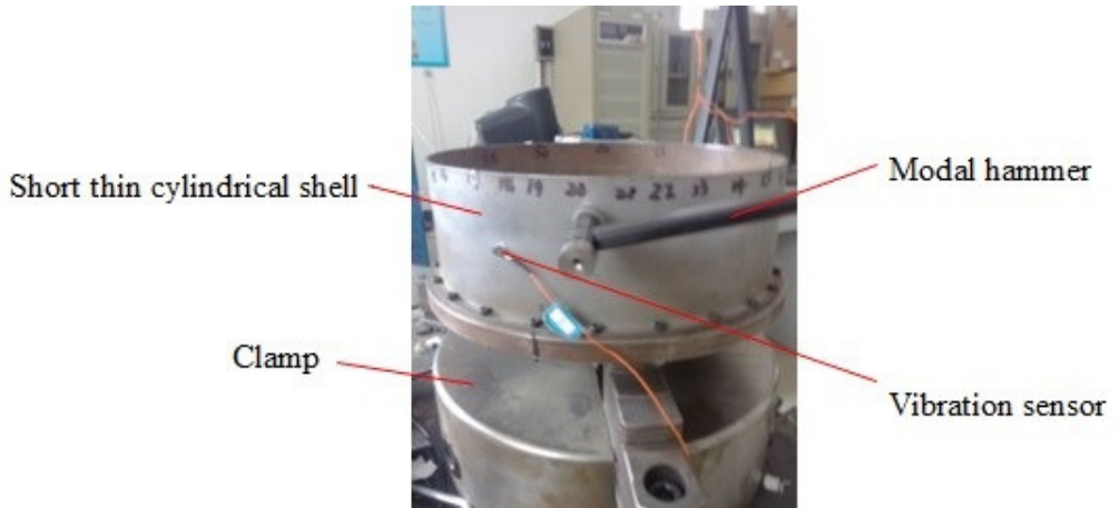
Fig. 6. Impact measurement system for modal of cantilever circular cylindrical shells
