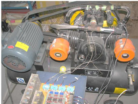
**Fig. 2.** Reciprocating compressor test platform
