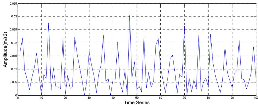
**Figure 5.** Absolute value of residual error of wear fault of valve plate.
