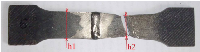
Fig. 8. Specimen No. 3 with clear evidence of necking
